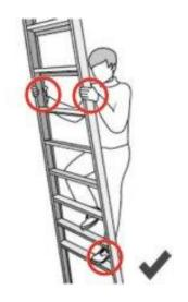
Maintain three points of contact with the ladder at all times.
