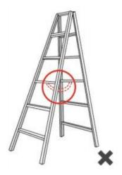
Do not use the ladder if the spreader bars do not have a locking device or mechanism.
