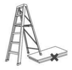
Place the ladder on stable and level ground. DO NOT place it on an uneven surface.
