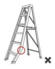
Do not use the ladder if it is bent or damaged.
